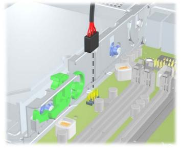
Figure 6-37 Disconnecting the Media Card Reader 1394 Cable
